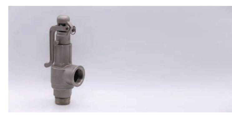
**Pressure relief valve** - A spring-loaded pressure relief valve which is designed to open to relieve excess pressure and to recluse and prevent the further flow of fluid after normal conditions have been restored. It is characterized by a rapid-opening 'pop' action or by opening in a manner generally proportional to the increase in pressure over the opening pressure. It may be used for either compressible or incompressible fluids, depending on design, adjustment, or application.
