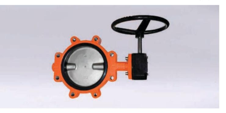
In a lugged connection the valve is fastened directly to the pipe flange by connecting the pipe flange with bolts to the valve body also drilled with threads.
