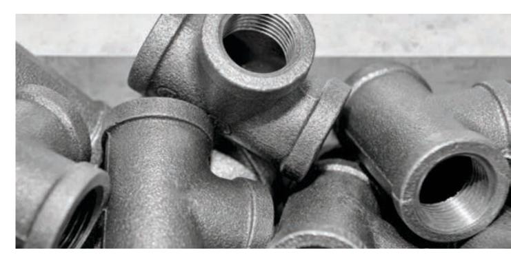
Threaded joints probably represent the oldest method of joining piping systems. Like Socket Weld fittings, threaded fittings are mainly used for small pipe diameters (Small Bore Piping); generally for piping whose nominal diameter is NPS 2 or smaller.
