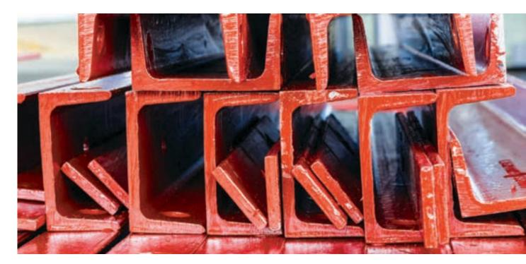
Steel channel has been classified into "C" and "U" types depending on its outlook. Hence there are two standards to show the channel dimensions - UPE & UPN. UPE is for the C channel steel with parallel flanges while UPN for the U channel steel with tapered flanges. You can find the size details in the specific type of channel steel like A36 steel channel. Bespoke channel dimensions are available.
