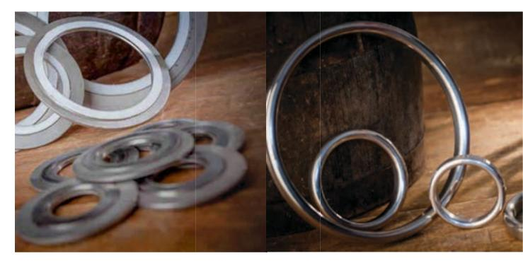
METALLIC GASKETS are fabricated from one or a combination of metals to the desired shape and size. Often used metallic gaskets are ring-type-joint gaskets (RTJ). They are always applied to special, accompanying flanges which ensure good, reliable sealing with the correct choice of profiles and material.
