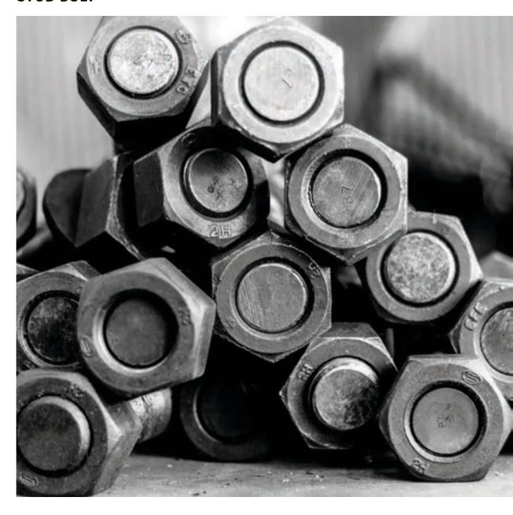
The quantity of bolts for a flange connection will be given by the number of bolt holes in a flange, diameter and length of bolts is dependent of flange type and Pressure Class of flange.
