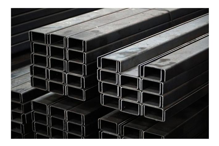
A U-channel is a long, thin metal strip shaped like the letter "U." It has a flat base (web) with two upright sides (flanges) running parallel to each other. U-channels are typically used for two main purposes:
