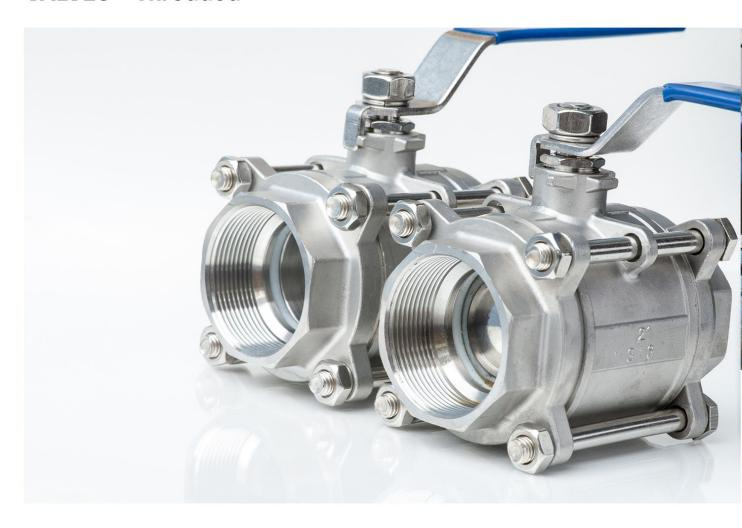
A threaded valve is a type of valve that uses threads on its ends to screw into pipes or fittings. This creates a tight seal that prevents leaks. Threaded valves are commonly used in plumbing applications, as well as in industrial and hydraulic systems. They are available in a variety of materials, including brass, stainless steel, and PVC, and can be used with a variety of fluids, including water, oil, and gas.
