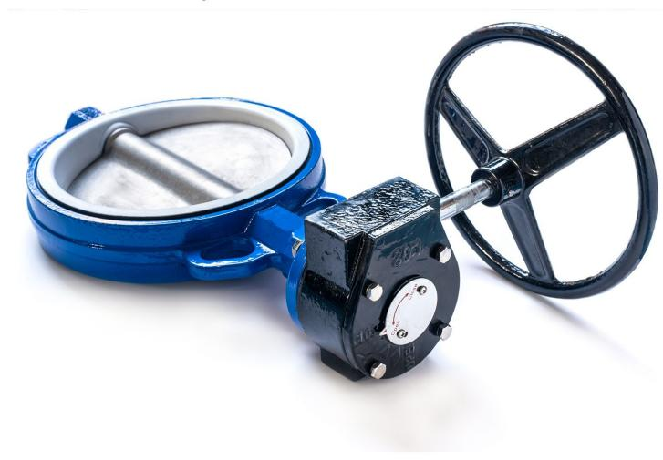
A wafer-style valve is a space-saving valve design that sits between two flanges on a piping system. Unlike flanged valves that have their own flanges for bolting on, wafer valves rely on the clamping force of the existing flanges in the pipeline to create a tight seal.
