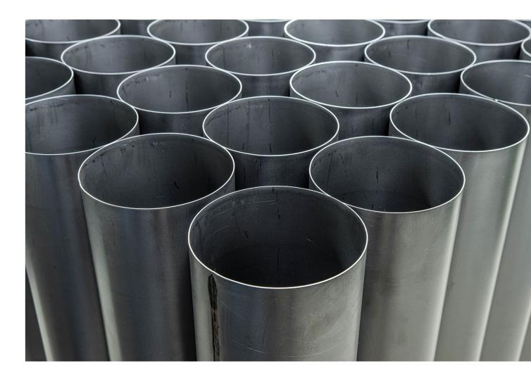
Welded pipe is a type of pipe created by forming a flat sheet of metal, typically steel, into a cylindrical shape and welding the seam shut. There are various welding techniques used to manufacture welded pipe, including electric resistance welding (ERW) and submerged arc welding (SAW).
