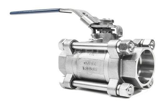
Socket weld valves offer a dependable solution for connecting pipes, particularly those with smaller diameters (typically NPS 2 or below). They excel in applications demanding high pressure and leak-proof connections. The valve features a socket-shaped end with a cavity where the pipe's smooth end is inserted. A fillet weld encircles the joint, creating a permanent and robust connection.
